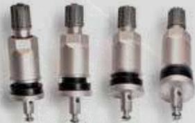
As for all other tire components, there are some particular storage recommendations for valves. Always protect valves from exposure to direct sunlight and contamination of oils, lubricants, fuels, solvents or other chemical substances.
