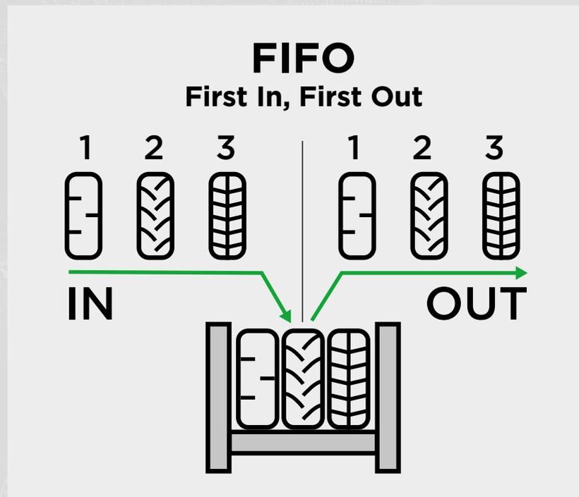
The best way to store your tires is in an upright position. This can be in single layers on a tire rack or shelf. Interlaced storage (fishbone method) is also possible, but avoid stacking your tires horizontally (stovepipe method), one on top of the other. Should this be impossible, limit the interlacing or stacking height to avoid that your tires are permanently deformed, especially at the bottom of the stacks, in addition to possible stability issues.
