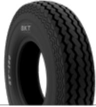
ST 180 is a tire developed for haulage applications with trailers and implements. Its specific tread pattern ensures a long tire life-cycle due to reduced wear. ST 180 is available in different versions: an "aramid belted" version ensures improved puncture resistance, while the "special" version provides high cut and chip resistance.
