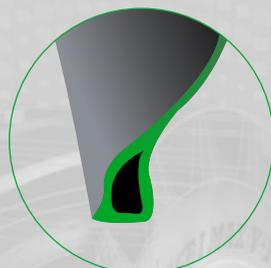
**Bead Protection System** for a more air-tight fitting on the rim
