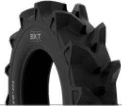
TR 173 is a tractor tire suitable for wet conditions and paddy fields. The special tread pattern provides outstanding self-cleaning properties in addition to reduced soil compaction thanks to a large contact area.
